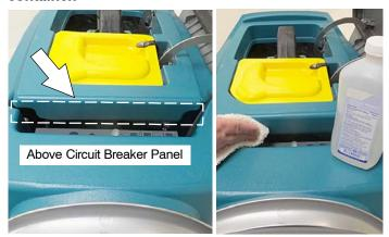
Gently bend or pinch the primer pen at center until the glass vial inside breaks. It will make a cracking sound. Rub primer pen on the clean recovery tank surface as shown. Allow primer to dry for 5 minutes before applying splash guard.
