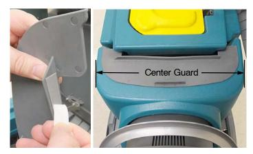
4. Hold the splash guard as shown and carefully adhere the guard to the primed surface. Firmly press the adhesive tape against the tank surface. Be careful not to press the center of the guard downward. The guard should lay flat on top of solution tank.
